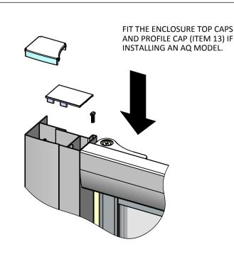
IF INSTALLING WITH AN ELLA SIDE PANEL, YOU WILL NEED TO NOTCH THE CORNER POST TOP CAP BEFORE FITTING.
