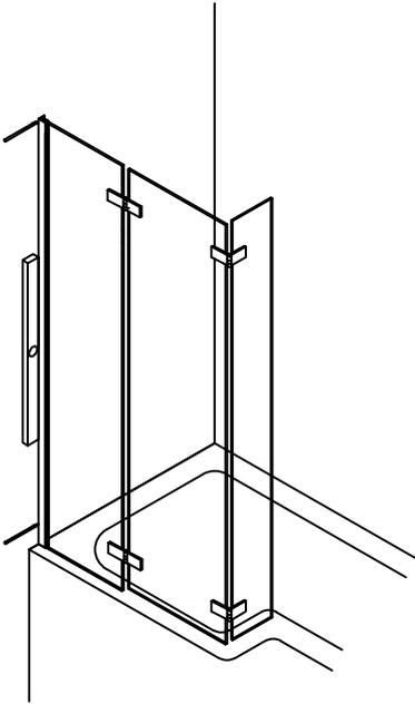
2. PUT THE WALL POST ONTO THE FIXED PANEL, WITH THE HELP OF ANOTHER PERSON PLACE IN POSITION ON THE BATH. USING A SPIRIT LEVEL MARK THE POSITION OF THE WALL POST ON THE WALL WHERE IT WILL BE FIXED.
