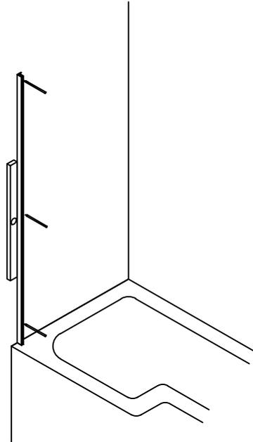
3. REMOVE THE SCREEN AND WALL POST FROM THE BATH, TAKE THE WALL POST AND PUT BACK INTO POSITION, USING A SPIRIT LEVEL TO ENSURE THAT THE POST IS PLUMB MARK THE POSITION OF THE 3 FIXING HOLES.
