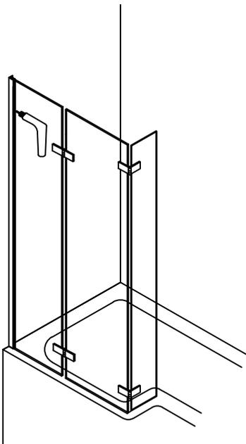
5. WITH THE HELP OF ANOTHER PERSON PLACE THE ASSEMBLED SCREEN INTO POSITION . MARK THE POSITIONS FOR THE 3 SIDE FIXINGS (SLIGHTLY OFFSET FROM THE WALL FIXINGS SO YOU CAN FIX THE COVER CAPS)ENSURE YOU DRILL THROUGH INTO THE FIRST PART OF THE HOLLOW BOX SECTION OF THE ALUMINIUM PROFILE ON THE FIXED SCREEN BEING CAREFUL NOT TO GO THROUGH THE OTHER SIDE(DO NOT DRILL INTO THE GLASS SECTION). DRILL THROUGH USING A 3.2 mm BIT AND FIX USING THE 10mm SELF TAPPING SCREWS.
