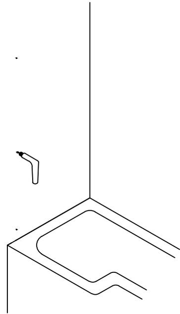
4. REMOVE THE WALL POST AND DRILL WHERE MARKED FOR THE WALL FIXINGS. REPLACE THE WALL POST AND SECURE INTO POSITION.
