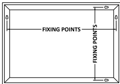
Measure the distance between the two holes on the wall and drill holes for wall plugs ensuring the holes are drilled level.
