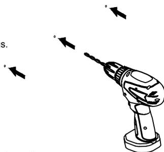
Fit the wall plugs into the wall and fix using screws.
