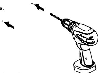
Fit the wall plugs into the wall and fix using screws.
