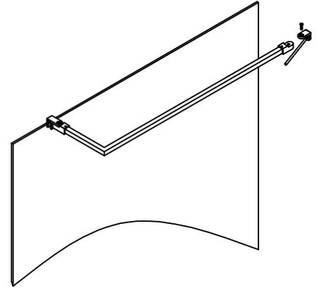
REMOVE THE END OF THE FIXING BRACKET BY UNDOING THE RETAINING SCREW.
