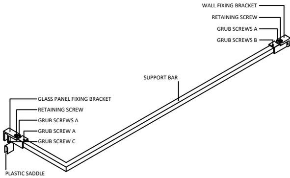
THE UNIVERSAL ARM CAN BE USED IN DIFFERENT POSITIONS BY REMOVING THE END FIXING BRACKETS AND CROPPING TO SIZE.
