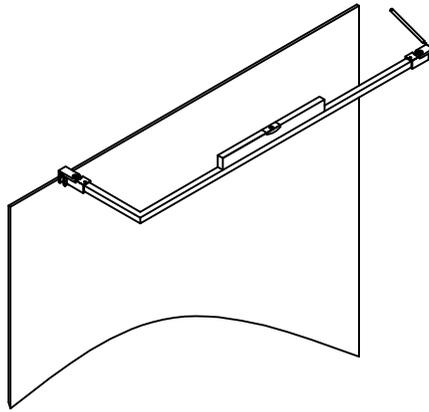
PLACE THE PLASTIC SADDLE IN THE GLASS PANEL FIXING BRACKET AND PLACE INTO POSITION ONTO THE PANEL AS SHOWN.
