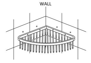
Using the appropriate drill bit, and drill the wall for the wall plugs **Note!** Alternative fixings may need to be used depending on wall type.
