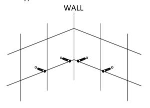
Place the screws through the screw cups and use a hand held screw-driver to fix in position.
