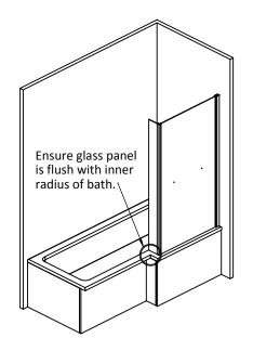
Slide the wall profile (2) onto the screen. Sit the screen onto the bath and adjust so the short glass panel butts upto the inside radius of the bath. Mark the position of the wall profile (2) with a pencil.
