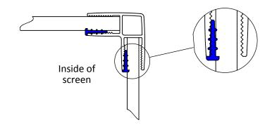
Insert the vertical wedge seal (6) into the corner post as shown above. Push the seal down the length of the corner post. A wooden block can be used to aid fitting. Trim off any surplus seal at either end, so its level with the profile.
