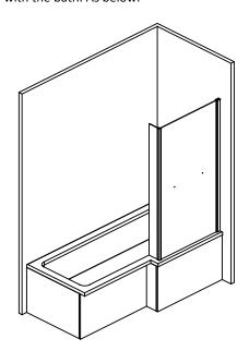
From the inside of the bath screen make a pencil mark on the wall profile approximately 100mm from the top and the bottom.
