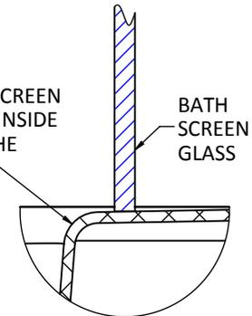
INSERT THE GLASS PANEL INTO THE WALL PROFILE (TAKE CARE AS THE GLASS IS NOT FIXED AT THIS POINT).
