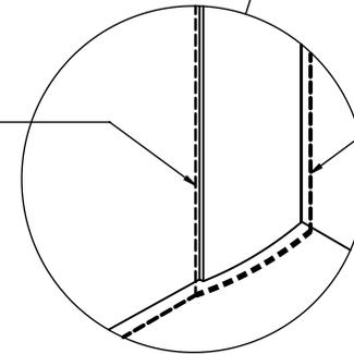
EXTERNALLY SILICONE SEAL THE WALL PROFILE WHERE IT MEETS THE WALL AND ALONG THE BOTTOM WHERE IT MEETS THE BATH. ALL IN A CONTINUOUS FULL BEAD.
