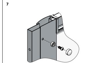
WHEN THE FRAME IS READY TO BE FIXED DRILL THROUGH THE HOLES IN THE GLASS PROFILE WITH A 3mm DRILL BIT.
