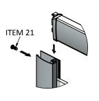
ONCE THE TOP & BOTTOM TRACKS ARE IN PLACE USE ITEM 21 TO SECURE THE FRAME TOGETHER.
