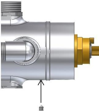
Tighten the chrome retaining collar by turning it clockwise. Tighten the collar to 17 Nm and then replace the grub screw to ensure the collar does not come loose.
