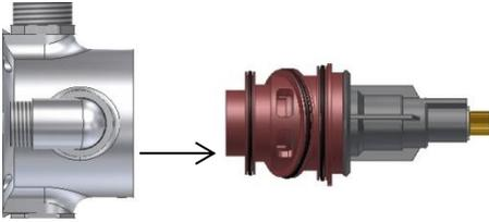
Pull the cartridge from the valve body.
