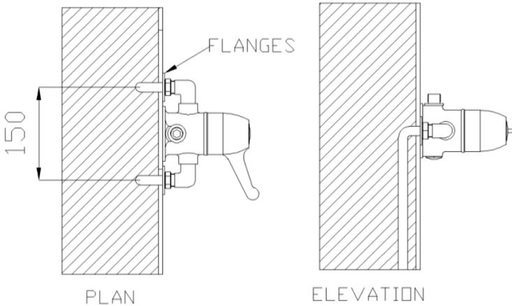
1. Make sure the pipes are at the correct centres as shown above.
