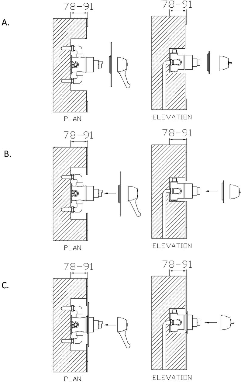
1. Make sure the pipes are at the correct centres. A cavity is required within the depth shown on the diagram. The depth depends on how far you want the valve protruding from the finished surface. The dimension is from the finished surfaced.
