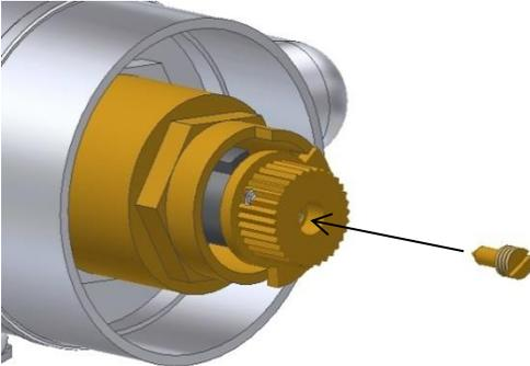
Once the stabilised outlet temperature is correct replace the spindle sealing screw.
