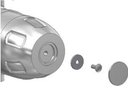
Turn the handle clockwise until it stops in the off position. Remove the cap and undo the screw. Remove the screw and washer. Put these in a safe place. The handle can now be removed.
