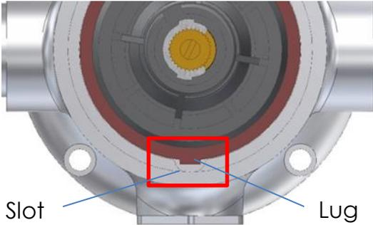
Place the new cartridge in the valve as in the diagram.
