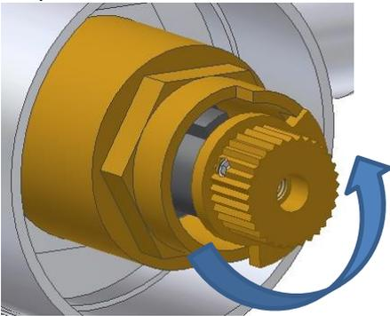
The water should now have stopped coming from the outlet. This means the Off position has been set and the max hot temperature can be set.
