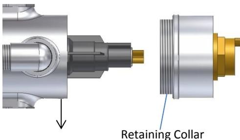
In order to remove the Chrome Retaining Collar you must remove the M5 grub screw that holds it. This is positioned at the underside of the body.
