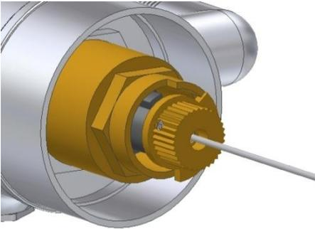
In order to calibrate the valve to the correct outlet temperature please place a 3mm flat bladed screw driver into the spindle. Locate the calibration screw slot inside and turn anticlockwise to increase the temperature or clockwise to reduce it. Allow the valve to stabilise after every adjustment and measure the outlet temperature.
