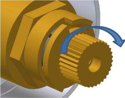
Place the Brass Stop Ring back on the spindle one serration anticlockwise of the Stop Ring. Turn the Brass Stop Ring clockwise until it reaches the Stop Lug. If the water still has not shut off repeat the step until it does.
