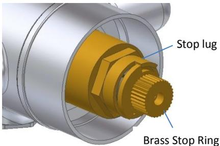
When the handle is removed the Brass Stop Ring will be revealed. This should be tight against the Stop Lug in the Off position. There should be no flow of water.
