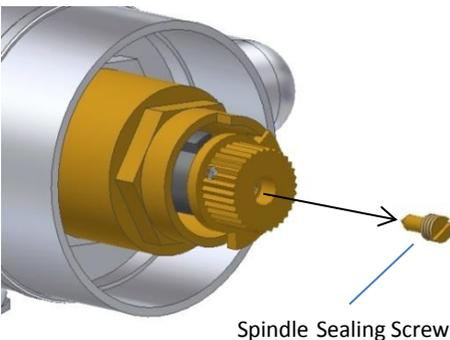
If the water is not the correct temperature, please use a small screw driver to remove the spindle sealing screw. This is located inside the spindle hole.
