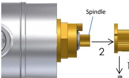
In order to stop the flow of water the Brass stop Ring position must be reset. To do this, remove the M4 grub screw holding the Brass Stop Ring in position. Then remove the Brass stop Ring.
