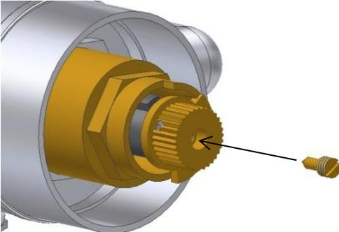
Once the stabilised outlet temperature is correct replace the spindle sealing screw.
