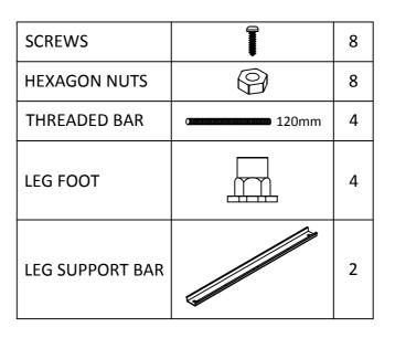
1. Fix leg support bars to the base of the Bath using screws (x8). PLEASE NOTE: the base board is encapsulated in the base of the bath.
