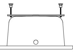
3. Adjust the height of the bath feet to match the bath panel height before installing the bath.
